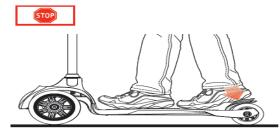
For controlled stops, apply the brake by stepping on the rear fender brake. It's recommends you practice applying the brake in an open area free from obstructions before riding your scooter around others
