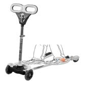
For controlled stops, apply the brake by stepping on the front fender/brake, It's recommends you practice applying the brake in an open area free from obstructions before riding your scooter around others
