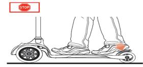
For controlled stops, apply the brake by stepping on the rear fender brake. It's recommends you practice applying the brake in an open area free from obstructions before riding your scooter around others
